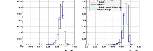
For CMS type crystal calorimeter an effect on EM shower from gamma-, electro- nuclear interactions was identified as a shift of peak energy deposition for 0.5%. In Geant4 10.0 these interactions are simulated with the Bertini cascade and neutron yield from gamma-nuclear interaction decreases compare to Geant4 9.6. This provides a shift of peak position of energy deposition for 0.2%.
