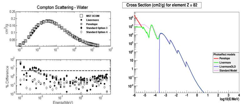
Main Geant4 gamma processes were revised and common approach was implemented for the Compton scattering and photo-electric effect:
