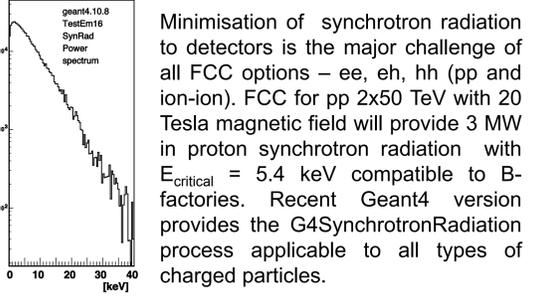
Minimisation of synchrotron radiation to detectors is the major challenge of all FCC options – ee, eh, hh (pp and ion-ion). FCC for pp 2x50 TeV with 20 Tesla magnetic field will provide 3 MW in proton synchrotron radiation with  $E_{critical} = 5.4$  keV compatible to B-factories. Recent Geant4 version provides the *G4SynchrotronRadiation* process applicable to all types of charged particles.
