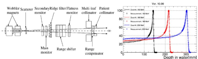
Methods of usage of proton and carbon beam for cancer treatment have been established in recent decade in Japan. HIBMC facility provides high quality beam allowing to measure of Bragg peak position in water with accuracy 0.1 mm.
