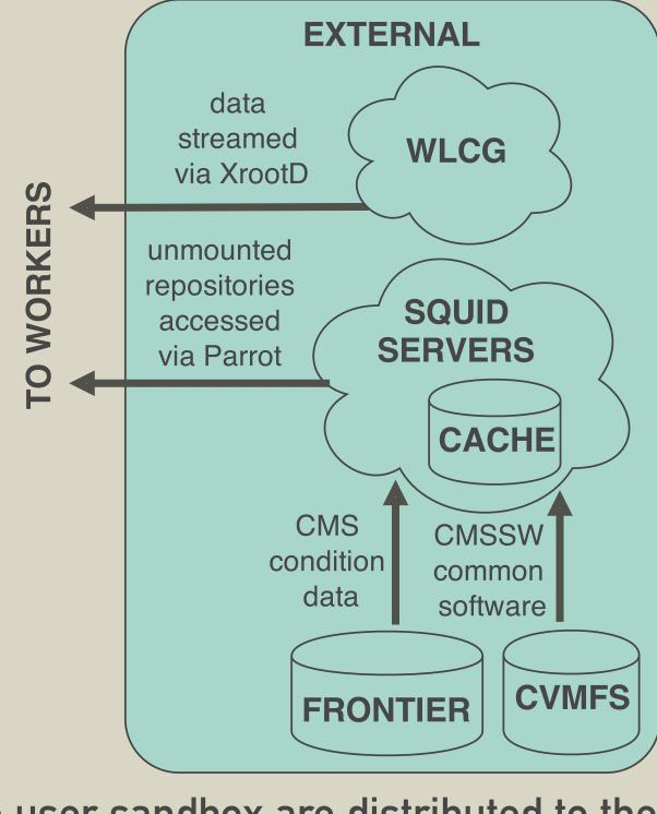
Job scripts and the user sandbox are distributed to the worker via WQ. The CMS software environment is mounted via the CernVM File System (CVMFS) and Parrot. Data is staged via Chirp or streamed via XrootD for local data storage and streamed via XrootD for access to the CMS wide-area data federation. CMS condition data is provided via Frontier. Outputs are transferred via WQ or an optional Chirp server.
