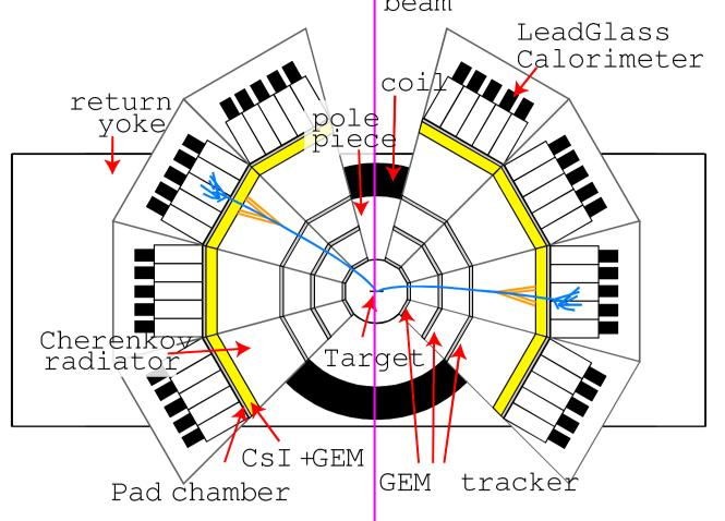
The J-PARC E16 spectrometer consists of GEM trackers, Cherenkov counters, and LG-calorimeters.
