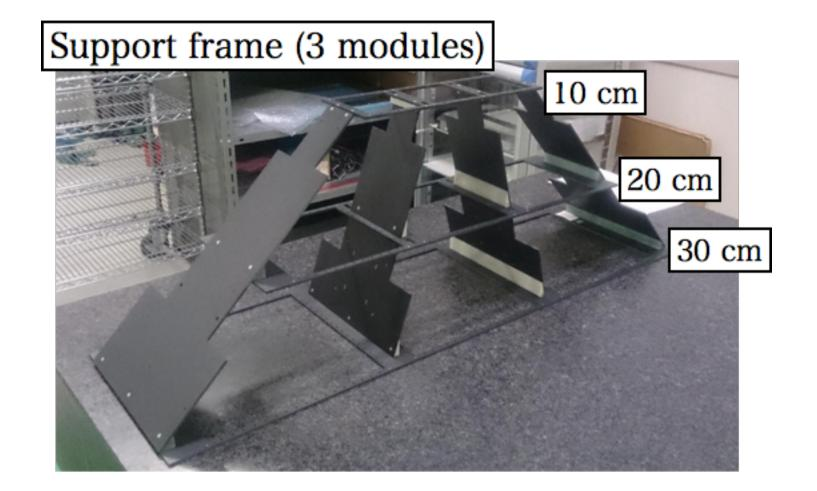
One module has 3-layers of GEM trackers (GTRs). The sizes of GTRs are 100 mm, 200 mm, and 300 mm, respectively.
