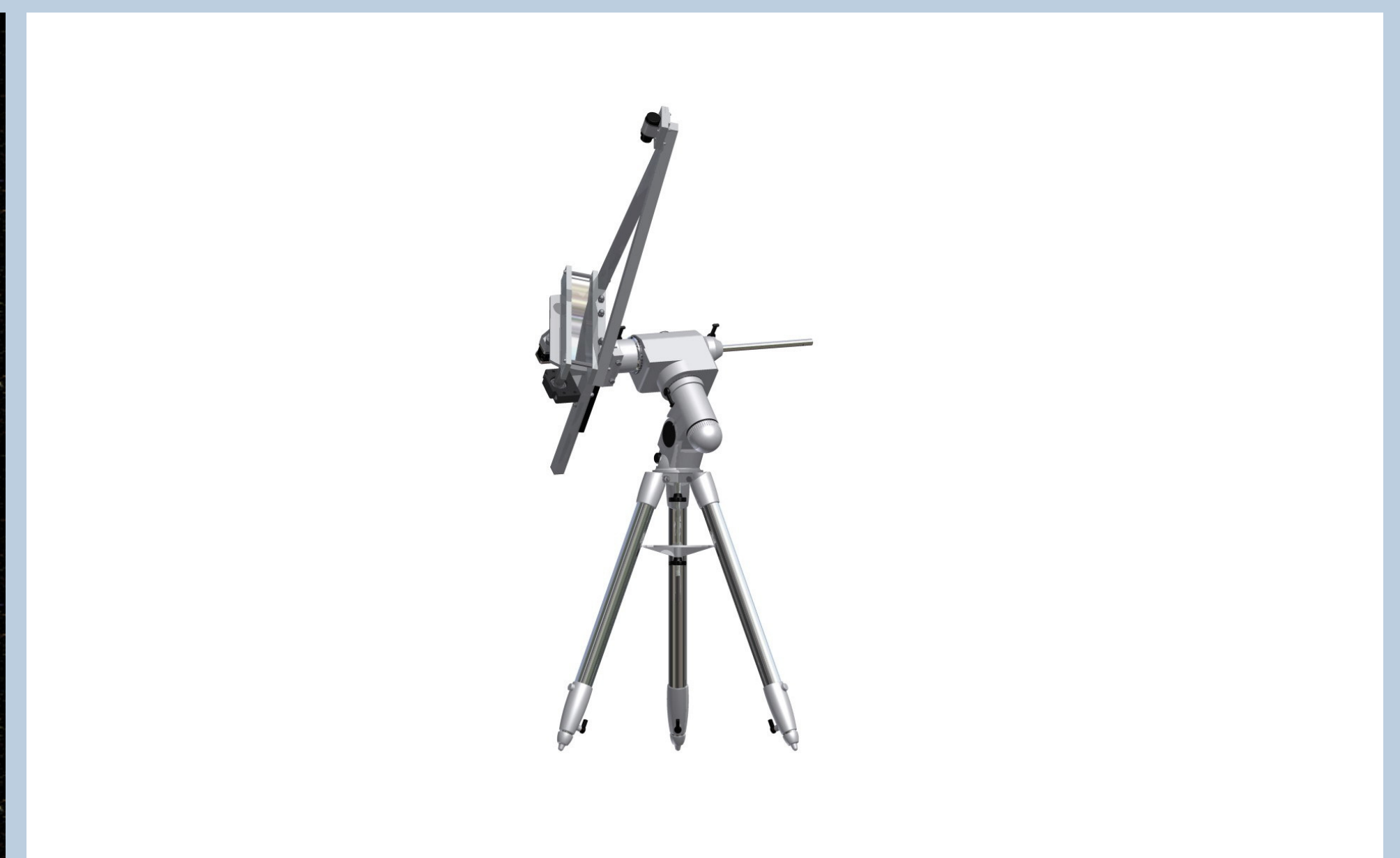
Figure 2: Parabolic strip telescope (left); Parabolic strip telescope on parallactic mount (right)
