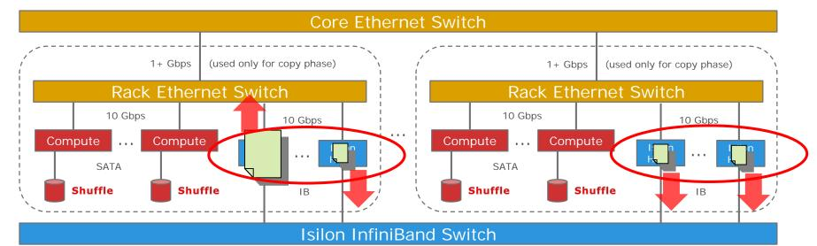
The number of compute and Isilon nodes can be adjusted independently to achieve the optimal ratio of compute and I/O bandwidth
