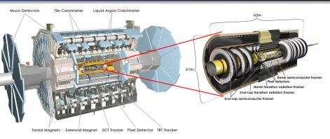
the ATLAS detector - almost full solid angle around the collision point coverage electromagnetic & hadron calorimeter, muon spectrometer
