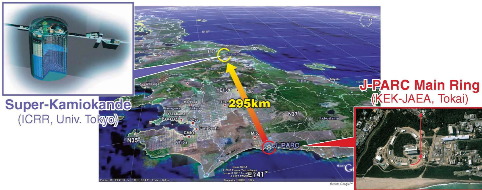
Overview of the T2K experiment, where a high intensity beam of \nu_\mu is created at Tokai and sent 300 km underground to the water Cherenkov detector Super-Kamiokande.
