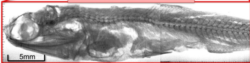
X-ray Image of a small dried sardine taken by a INTPIX4 sensor (3 images are combined).
