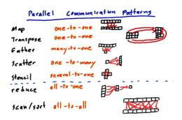
Illustrate one parallel patterns implementation on GPU: the stencil pattern using a heat equation solver algorithm.
