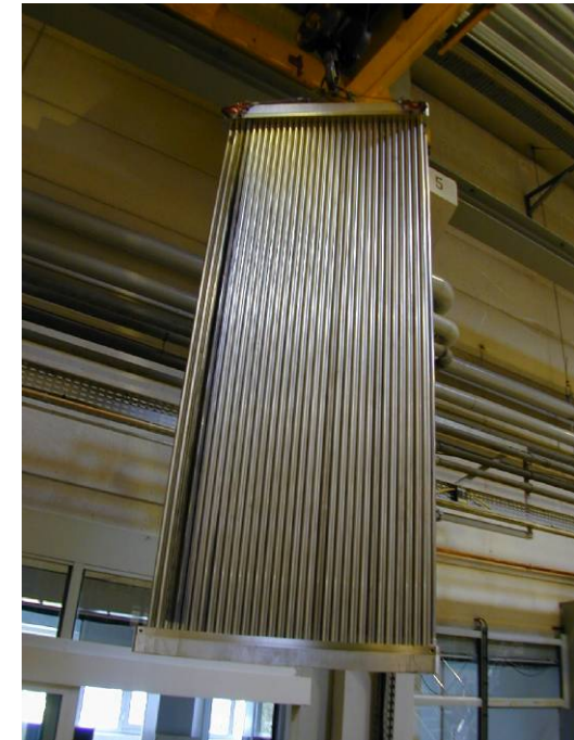
2m long, position-sensitive proportional counters for other time-of-flight experiments
