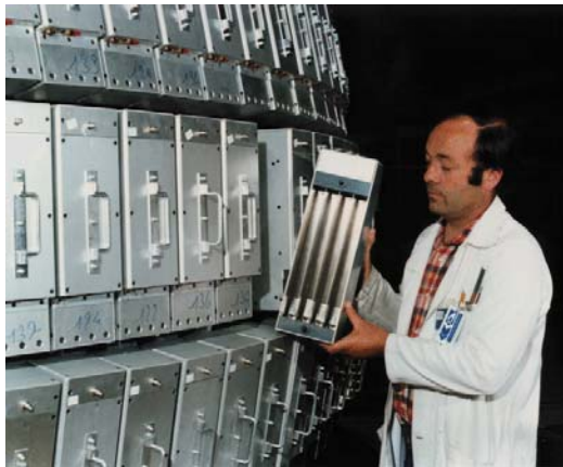
Beam-line IN6 (ILL, Grenoble): a time-of-flight spectrometer for quasi-elastic and inelastic scattering.
