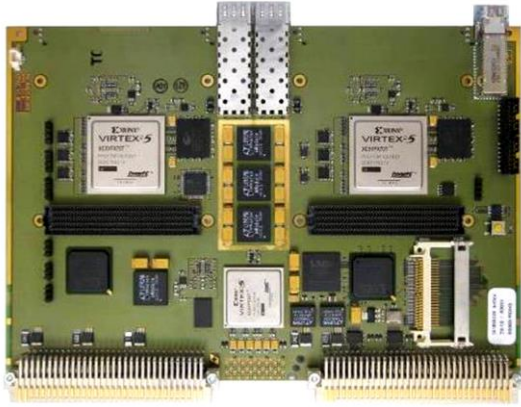
Modular BPM electronics for SLS (PSI)
