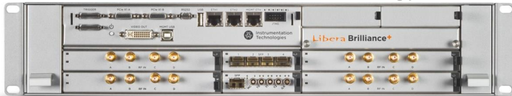
Commercial BPM electronics (Instrumentation-Technology)
