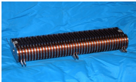
First wound 42-pole test coil
