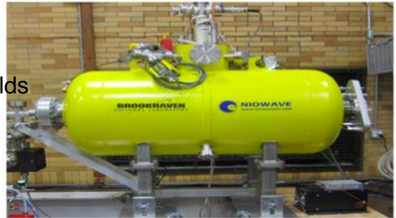
Figure 7: Cold test setup of the 1500 MHz cavity
