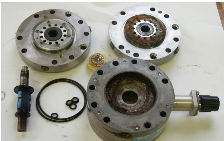
Corrosion due to demineralized water in the cooling system
