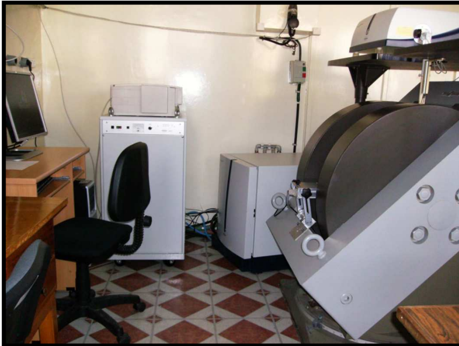
The EMX-plus (Bruker) X-band spectrometer with Varian E12 magnet (NIMP - CetRESav)
