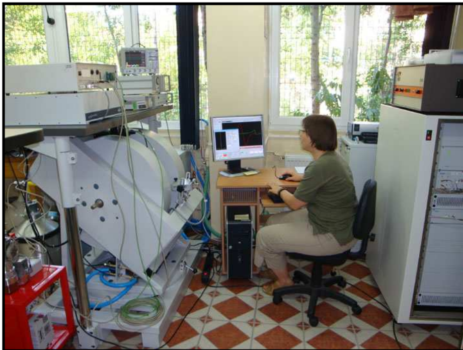
The Q-band CW ESR spectrometer ELEXSYS 500Q with E560 ENDOR unit
