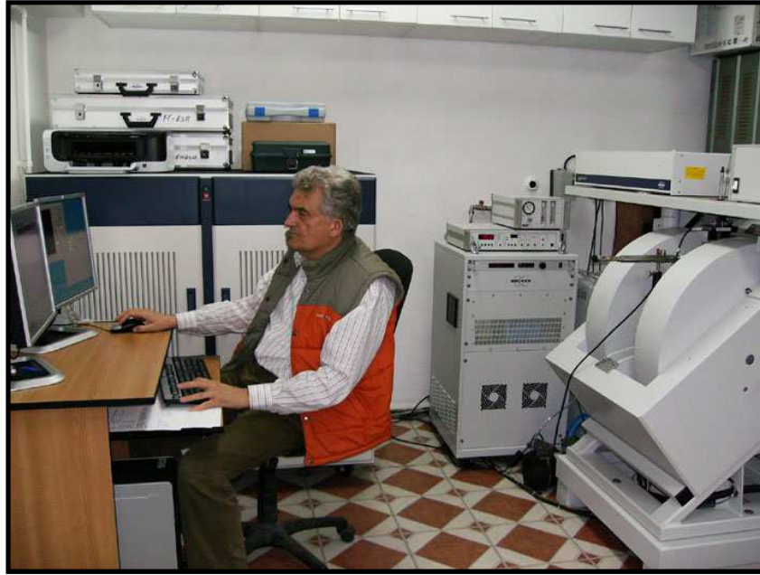
The X- band FT/pulse ESR spectrometer ELEXSYS 580 with E560 DICE ENDOR and E540 -400 pulse ELDOR
