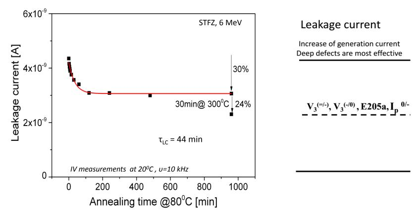
Contribution of defects at the leakage current:
