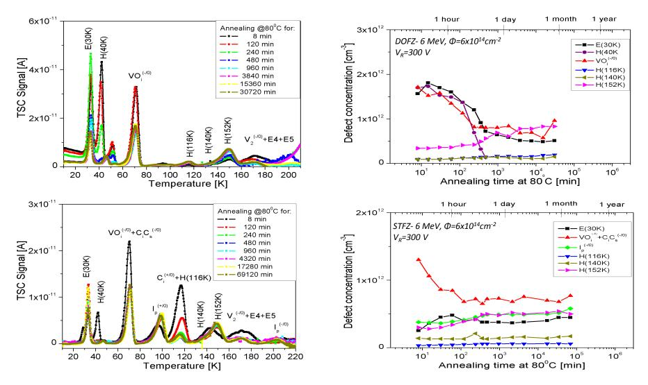
Elevated temperatures (up to 80 °C) are used to accelerate the effect of annealing to study the expected changes of the sensor performances over several years of room temperature equivalent time.
