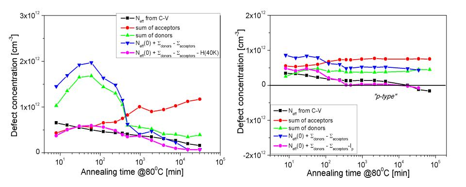
Change of N<sub>eff</sub>, with the annealing time (also with the aneealing temperature), well described by accounting only the E(30K), H(40K), Ip, H(116K), H(140K) and H (152K) – defects with unknown chemical structure
