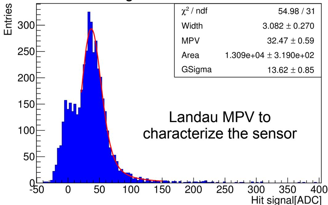
Epi100P, 23 GeV p,  $3 \times 10^{15} \text{ n}_{\text{eq}} \text{ cm}^{-2}$ , -800V, -20 C
