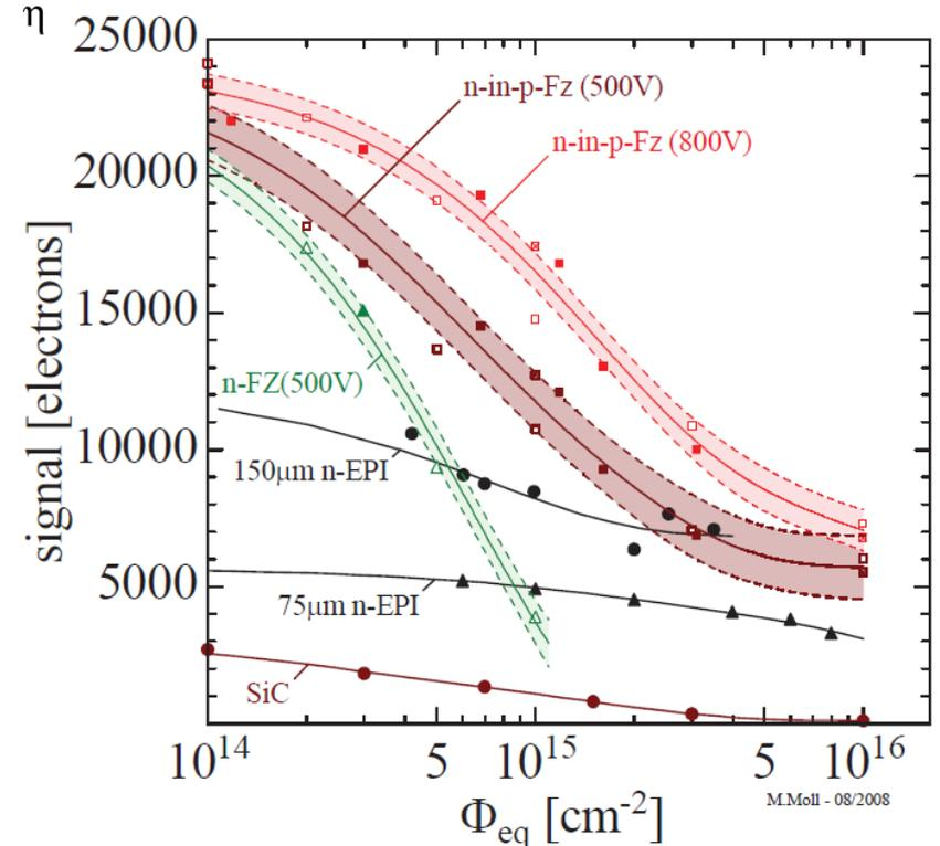
**Test beam of thin epitaxial strip sensors to determine material characteristics**
