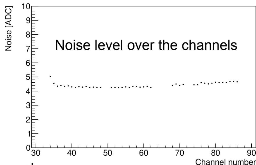
Mean and RMS of the noise over the channels
