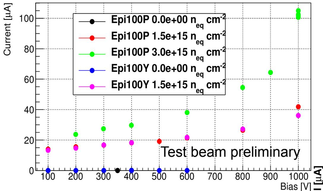
IV of both diodes and strips show a “soft breakdown”
