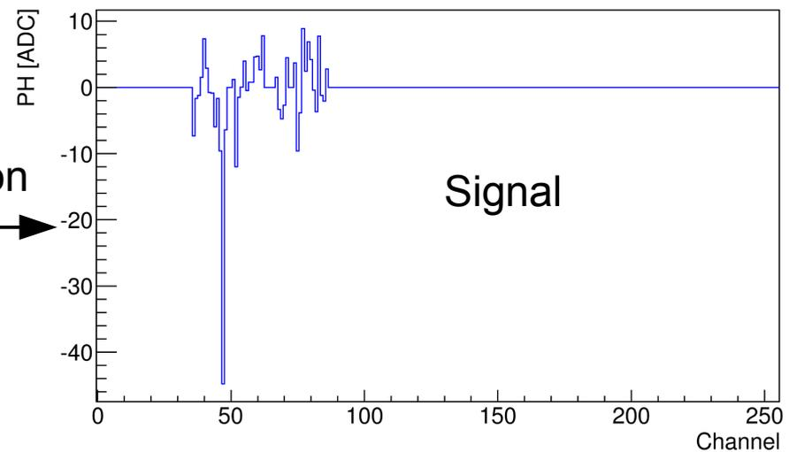
Epi100P, 23 GeV p,  $3 \times 10^{15} \text{ n}_{\text{eq}} \text{ cm}^{-2}$ , -800V, -20 C
