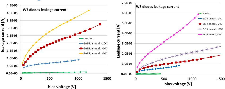
Leakage current increase is not linear with fluence. Increase with fluence in **smaller** due to degradation of multiplication
