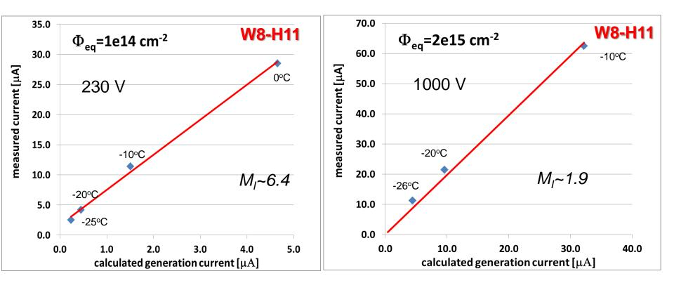
$$M_{I} = \frac{I_{leak}}{I_{gen}} = \frac{I_{leak}}{\alpha \cdot \Phi}$$
