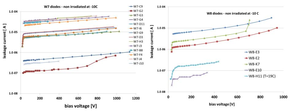
The current of the devices differ for almost 3 orders of magnitude for both wafers:
