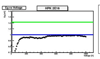
Sensors irradiated to  $1 \times 10^{15}$ ,  $5 \times 10^{15}$ ,  $1 \times 10^{16}$ ,  $1.5 \times 10^{16}$ ,  $2 \times 10^{16}$  n<sub>eq</sub>/cm<sup>2</sup> clearly lower E<sub>g</sub>  $\approx 1$ eV (blue line) than lower dose
