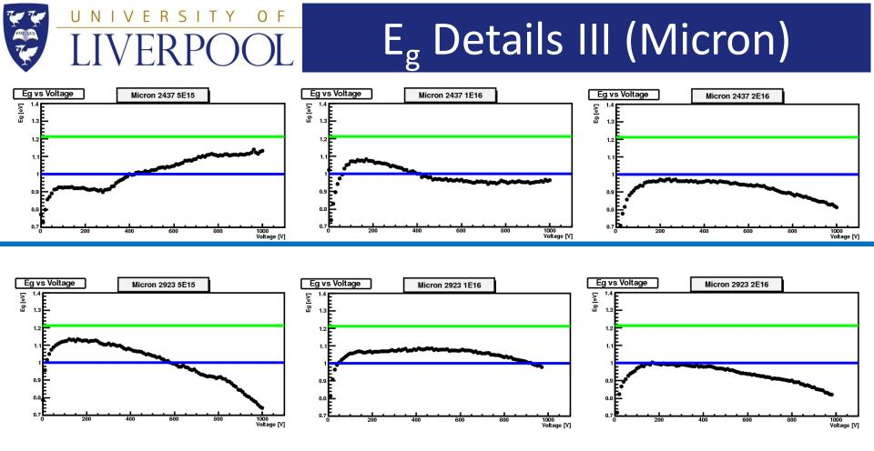
Also for Micron sensors (143 $\mu$ m (upper row) and 108 $\mu$ m (lower row) thick) E<sub>g</sub> for higher doses closer to 1eV (blue line) than to 1.2eV (green line)
