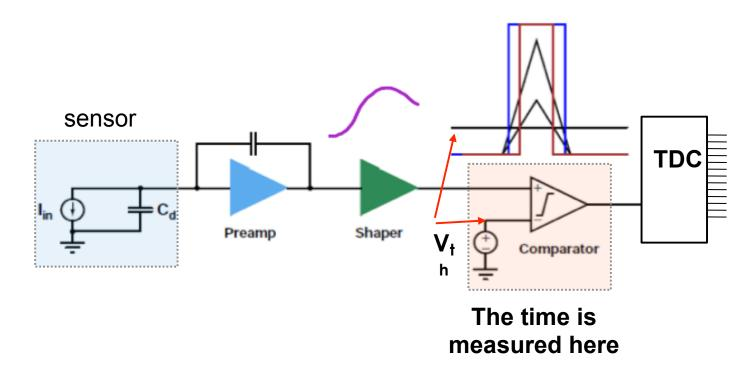
The timing capabilities are determined by the characteristics of the signal at the entrance of comparator and by the TDC binning:
