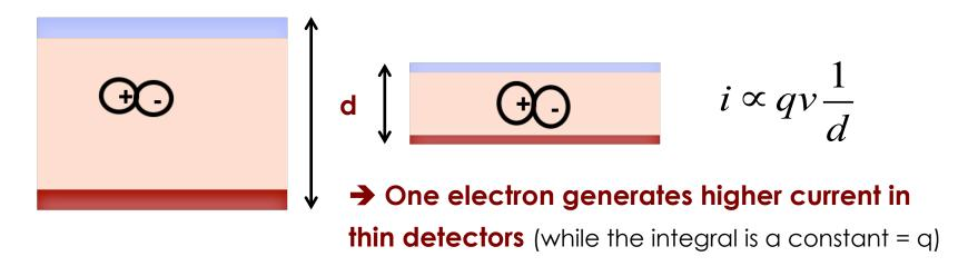
2) The initial current for a silicon detector does not depend on how thick (d) the sensor is:
