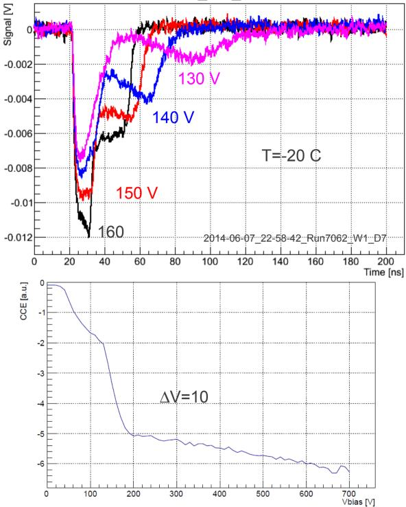
Waveforms for biases ranging from 130V-160V
