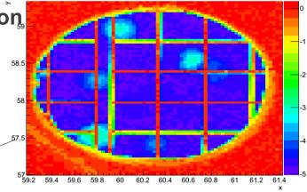
For integration times <80 ns, the charge is smaller at the "spots" than at the rest of the detector. We obtain a non-uniform multiplication map. Indeed, at the spots the holes seem to diffuse, while out of the spots they seem to drift (see next slide)
