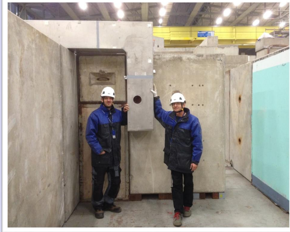
Proton shuttle conduit as seen inside the new irradiation area
