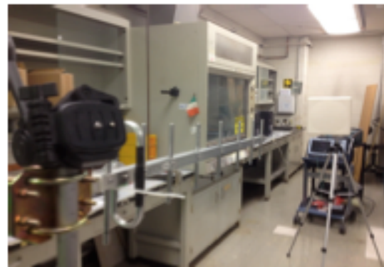
Figure 2: Apparatus for RF power transmission. Left figure shows the RF transmitter (14 dBi gain Yagi antenna) in the foreground, with the RF receiver (11 dBi gain patch antenna) at the far end. Right figure shows the power loss (dB) as a function of distance (m) from the source.
