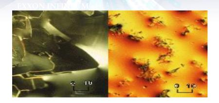
The photo shows large crystals formed at -13 °C and the same fuel treated with additives which lead to a significant reduction in crystal size.
