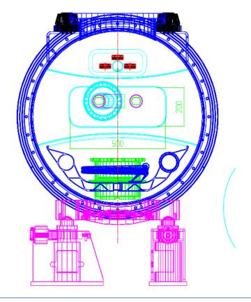
With respect to the previous version presented during the past meeting, the dimension of slots has been increased; only 2 slots of 4 m each one ,connected together by a passage of 500x 250 in the central region.
