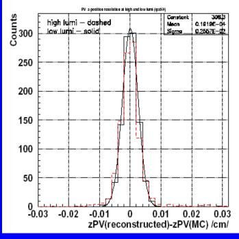
In this case 26µm. Very close to the best resolution with tracks!
