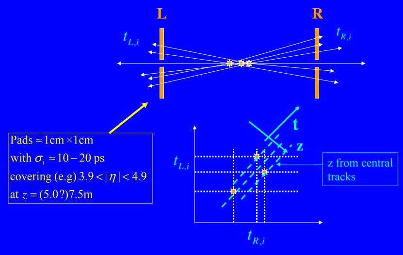
This can identify (in principle) interactions that have particles in both L and R detectors. <u>All are background for CEX!</u>
