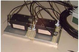
Resolution: 0.1 μm Range: 10 mm along two axes Repeatability: 1 μm Bandwidth: 0-100 Hz This slide courtesy of H. Mainaud-Durand
