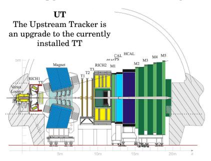
By removing gaps in the acceptance currently found in the TT, there is significant improvement to track reconstruction efficiency
