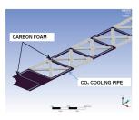
Evaporative CO<sub>2</sub> is used for cooling
