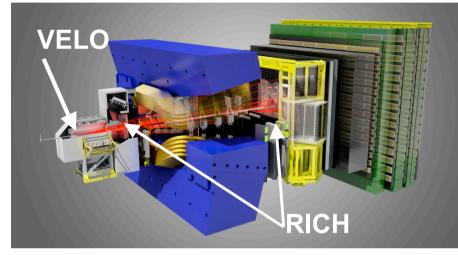
All measurements profit from the VELO for displaced vertices and the RICH for particle identification
