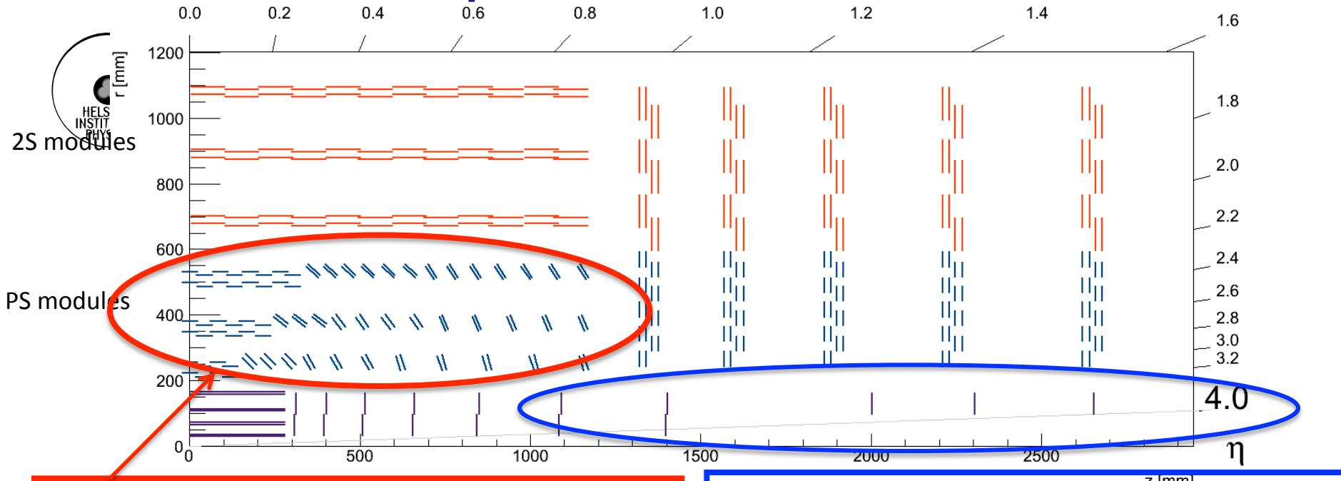
Tilted layout option under study: allows reduction of material and cost savings
