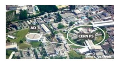
AD slows down antiprotons from near light speed to around 0.1c before sending them out for use.
