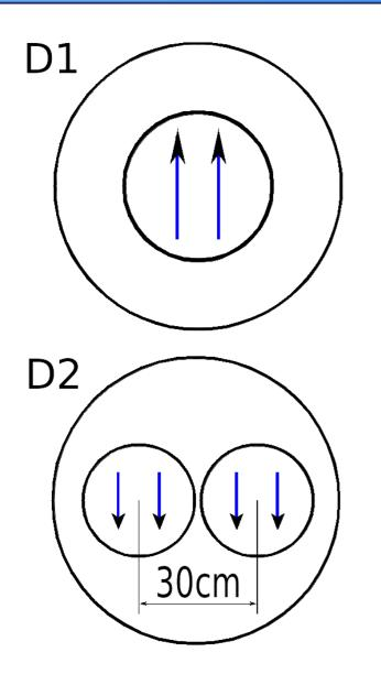
D1: shared by both beams, B= 5.74 T D2 separate dipoles, but magnetic fields have same directi D1
