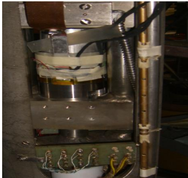
Compressive I_c test setup (LN2 testing)
