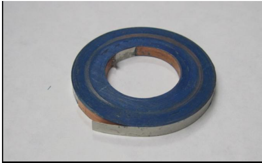
Pancake coil fabricated from 12mm wide SP 2G HTS
