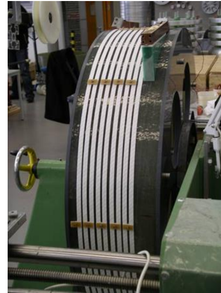
Roebel cable ready for testing at Siemens Corporate Technology, Germany.
