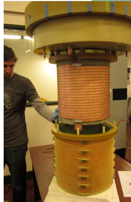
RRI – 1 MVA Transformer
