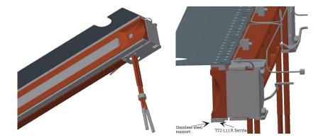
RF fingers are removed and their HOM damping functions are supposed to be supplied by TT2-111R ferrite blocks
