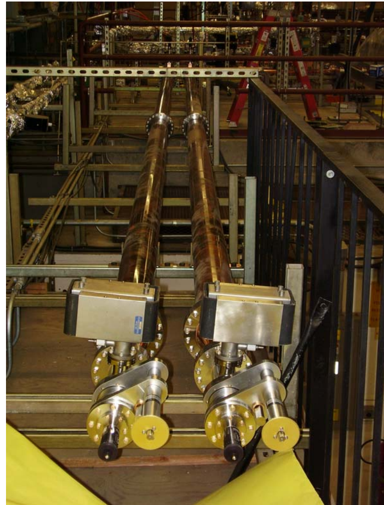
The ASTA pulse compressor with variable delay delay-lines( Miller cup)
