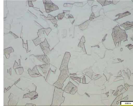
Metallography of CERN Copper before H<sub>2</sub> Fired (100x magnification) revealed an oxygen-free copper, cold worked with equiaxed, recrystallized grains that contained twinned regions. Very little contamination was observed.
