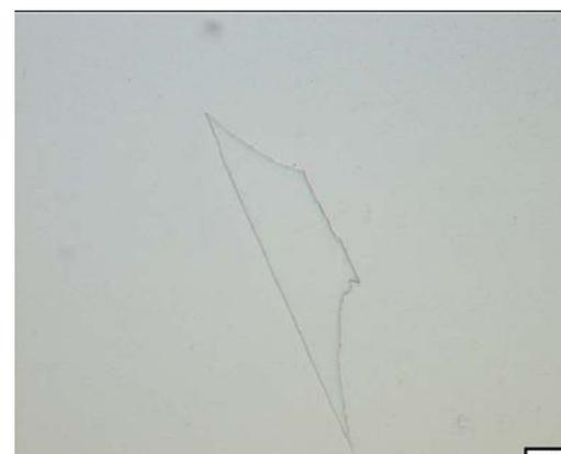
Metallography of CERN Copper after H<sub>2</sub> Fired (100x magnification) revealed large, coarse, well-defined crystals consistent with grain growth due to high temperature annealing. Classification is ASTM F68 Class 1 for type A (cross grain), B (within grain), & C (grain boundary).
