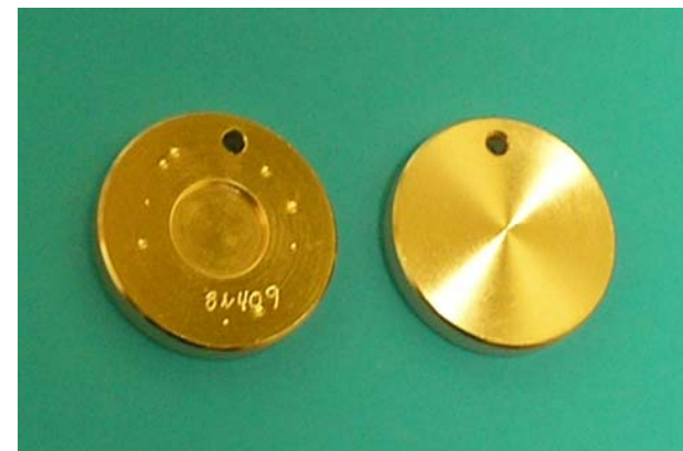
Top and bottom side of copper coupon H2 fired
