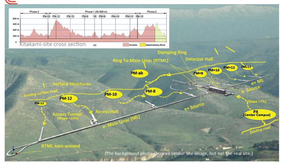
Need to establish the IP and linac orientation Then the access points and IR infrastructure Then linac length and timing
