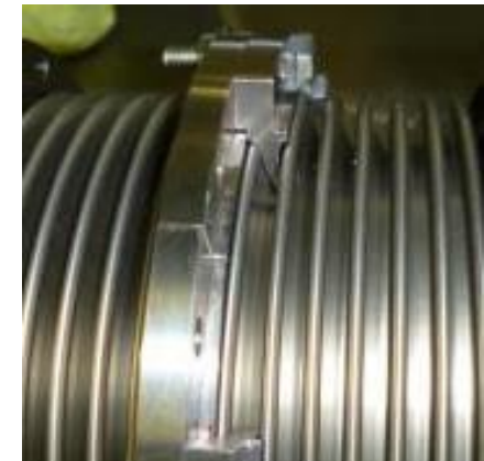
Convolution blocked – bellows not replaced
