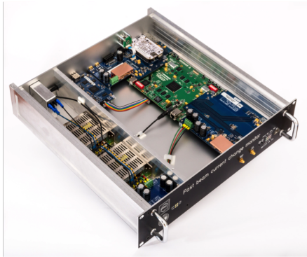
Figure 7: Picture of the operational FBCCM electronics box.
