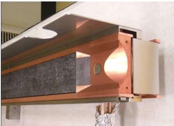
Figure 1: New TCSP carbon jaw with embedded BPM.
