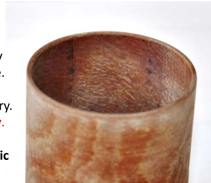
Sand blasted Bakelite tube after sparking
