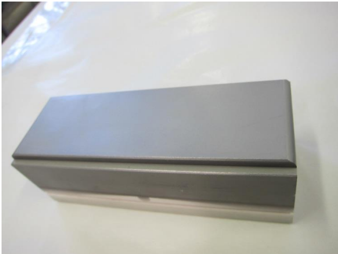
BN after coating (Ti 5um+NEG+Cu 2um+NEG)
