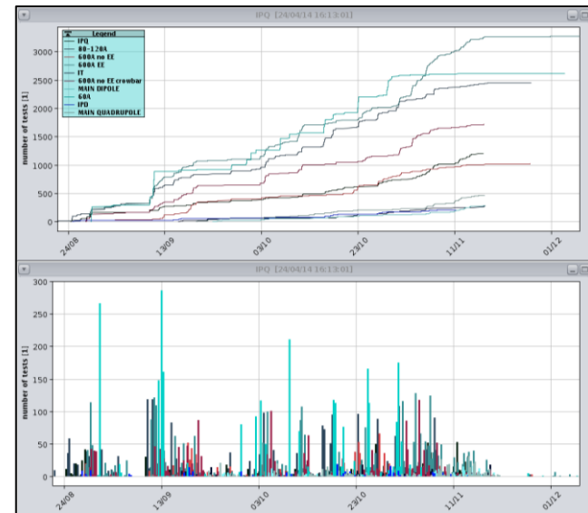
Cumulative number of powering test steps performed between August and December 2009 (divided per circuit type)
