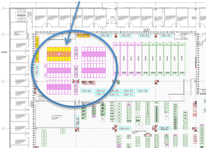
ORNL CACS - Cold Aisle Containment System
