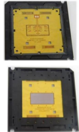
FPC prototype with mounted chip in TAB-70 technological frame
