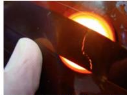
Figure 4. Non detected failure of a QH. As seen after dismantling during inspection of the QH.
