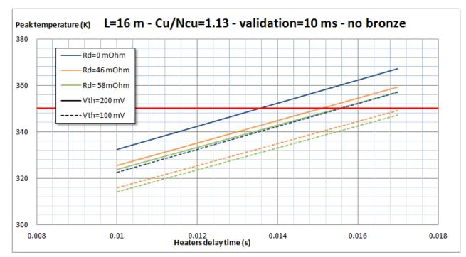
MT-23: MQXF hot spot temperature is **very close** to the conventional maximum of 350 K
