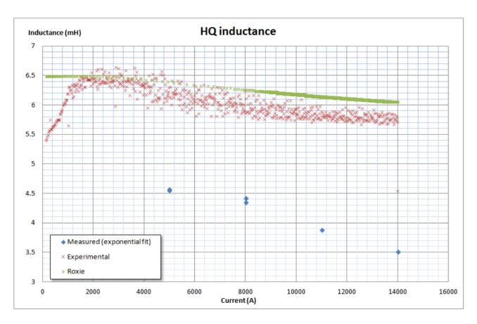
After a quench, during a discharge, magnets inductance appears **lower** than expected
