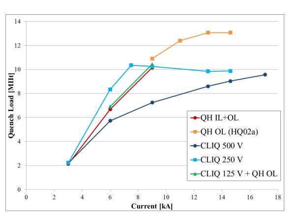
CLIQ performance during HQo2b tests are impressive: the whole magnet is almost totally quenched in less than 5-10 ms
