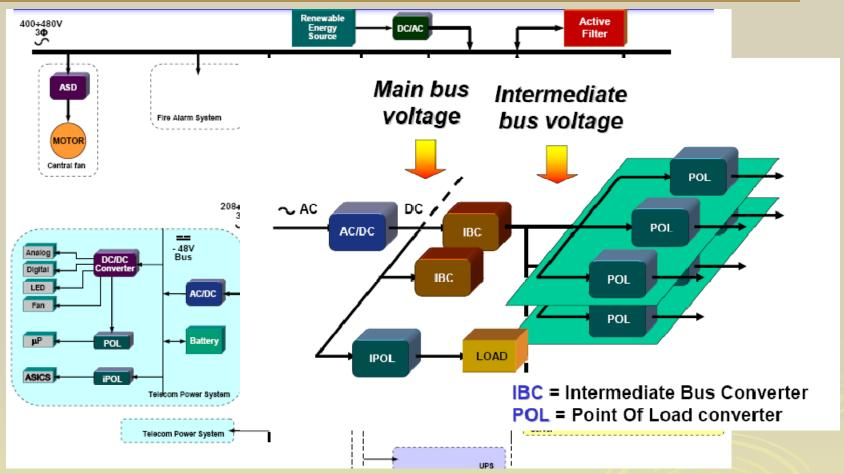
Conversion is performed in several stages for high efficiency and modularity. POL converters provide regulated power to the loads when needed.
