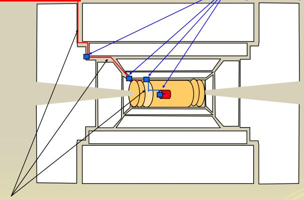
Current path from PS to module (or more seldom star of modules) and return. Cables get thinner approaching the collision point to be compatible with material budget.
